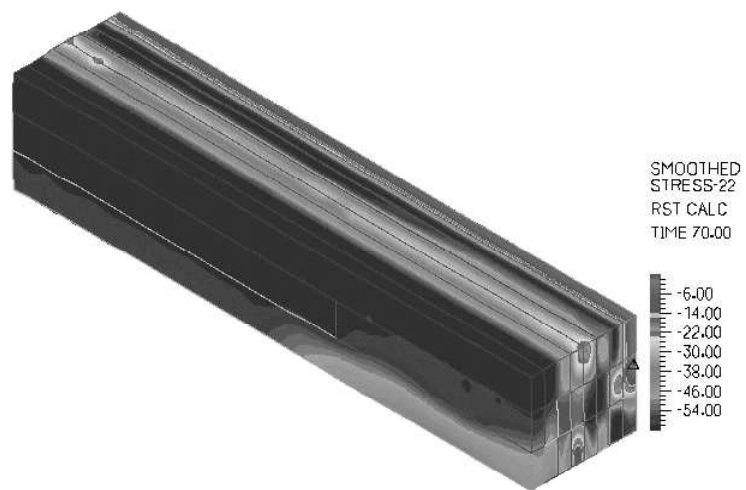
Figure 7.18. Sample finite element 1.55 in x 1.55 in x 5.00 in body. The top right corner of the cross-section has a very weak strand which carries little to no load.
