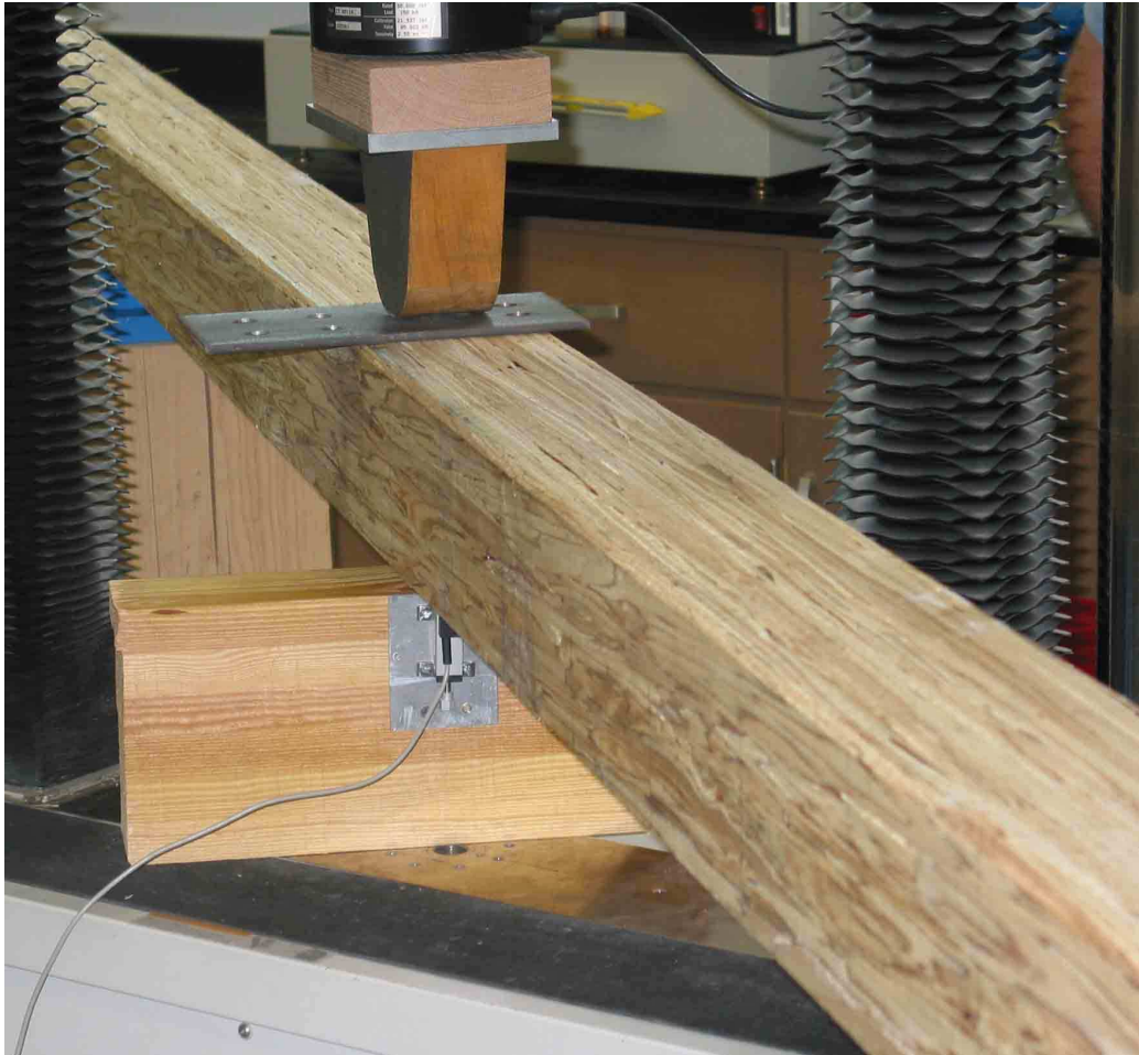
Figure 2.6. Bending test setup of a 5.25 in x 5.25 in x 16 ft experimental sample.
